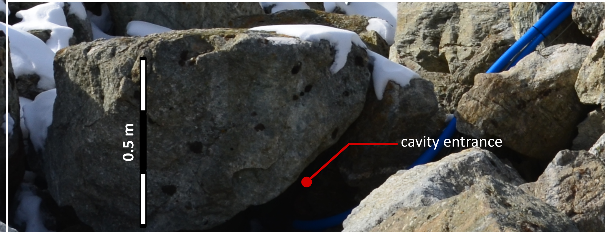
Fig. 3: The below-ground sensor array in a natural cavity, down to 3 m depth, located on a rock-glacier ridge. Installed sensors include: • wind speed sensors (Figs. 4, 5) • thermistors and hygrometers (Fig. 6)
