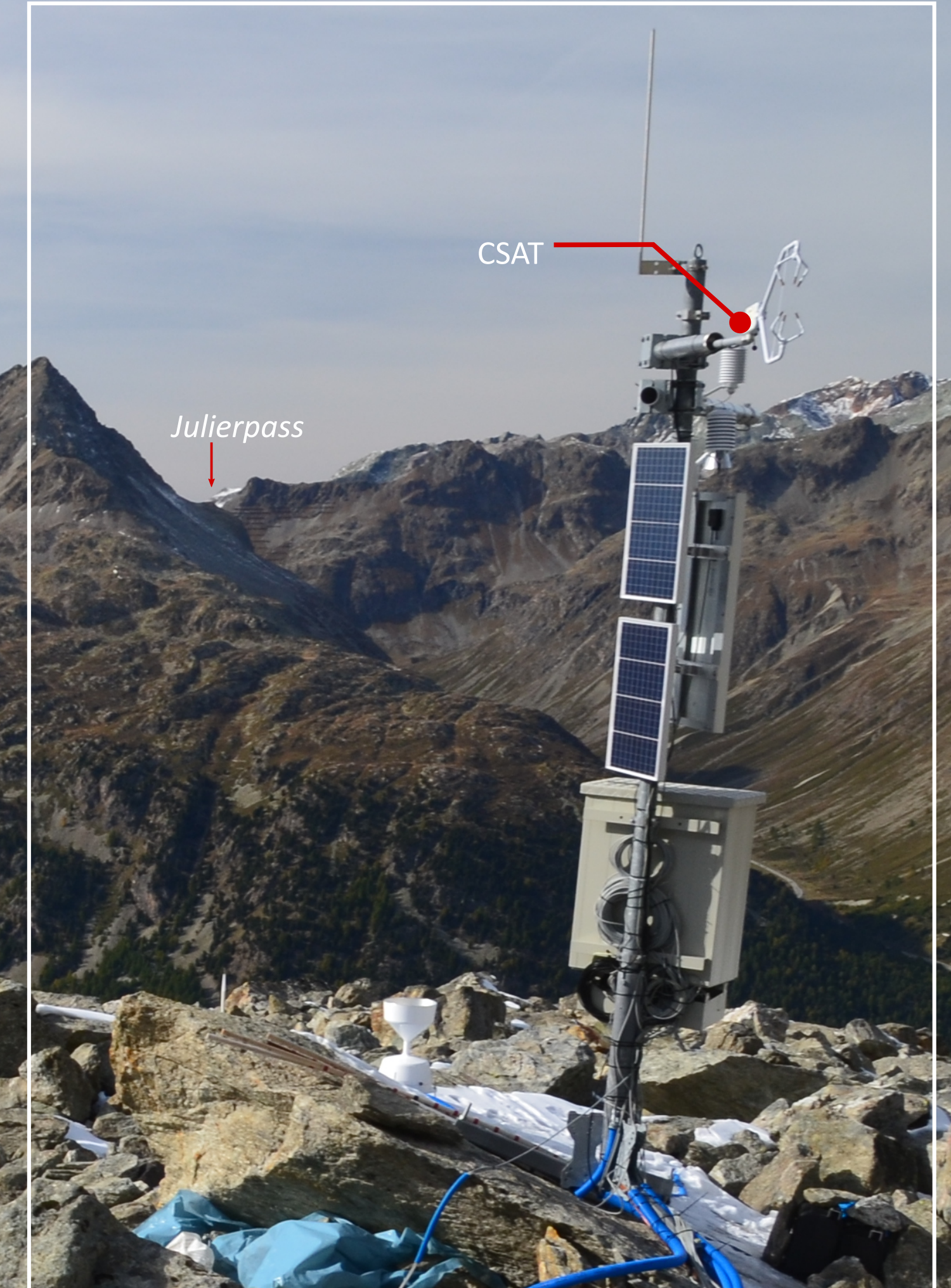
Fig. 2: The above-surface automatic weather station: meteo pylon with a CSAT sonic anemometer, a sonic ranger for snow height, hygrometer and pluviometer.
